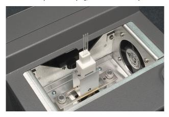
warm-up and cool-down cycling. Ramp rates from 0.1 °C/min. to 20 °C/min. (1-2-5 sequence) provide the flexibility needed for virtually any melt.
